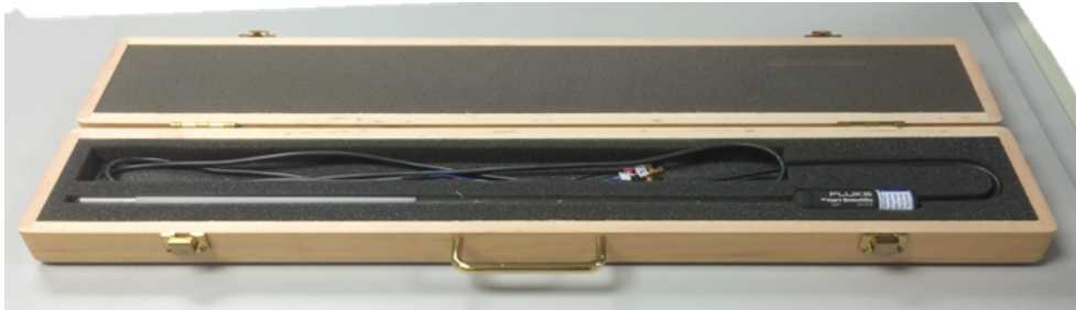
Figure 1: A glass SPRT with 405 mm probe length. The platinum wire is generally near the tip of the stem.
