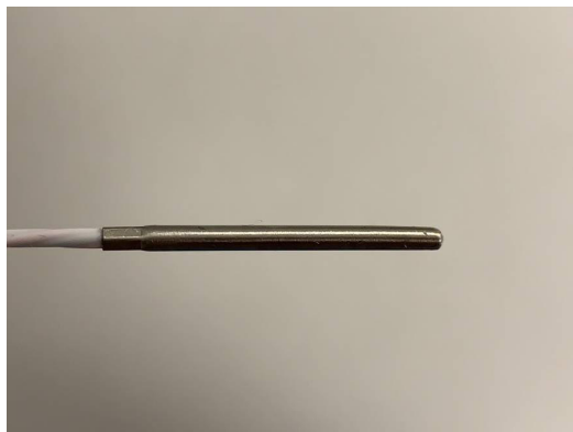
Figure 2: A capsule probe with 40 mm probe length.
